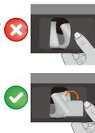
2 Inside Person: Ensure that the mat rod holder is correctly positioned with the small tag positioned outside the mat rod holder pocket.
