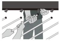
3 Inside Person: Take hold of the rod with both hands and maintain a steady grip until it is securely installed in the mat rod holder.
