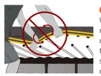
8 Outside Person: When you remove a rod from the mat, do not twist or rotate the mat edge as shown. This could cause serious injury or damage the trampoline.
