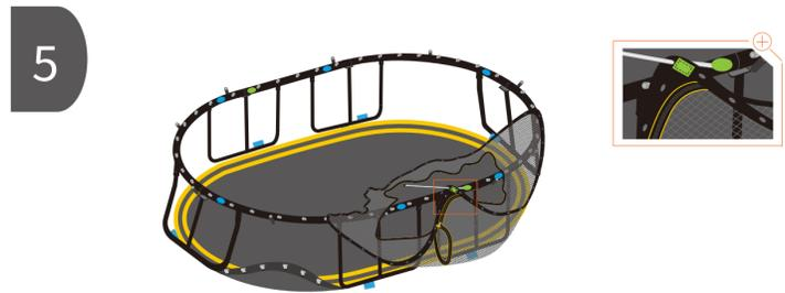
STOP NOTE - As you install the white mat rods into the mat rod sockets the net will become tight against the frame. Handle the net with care and be sure that it does not get caught or it may tear.
